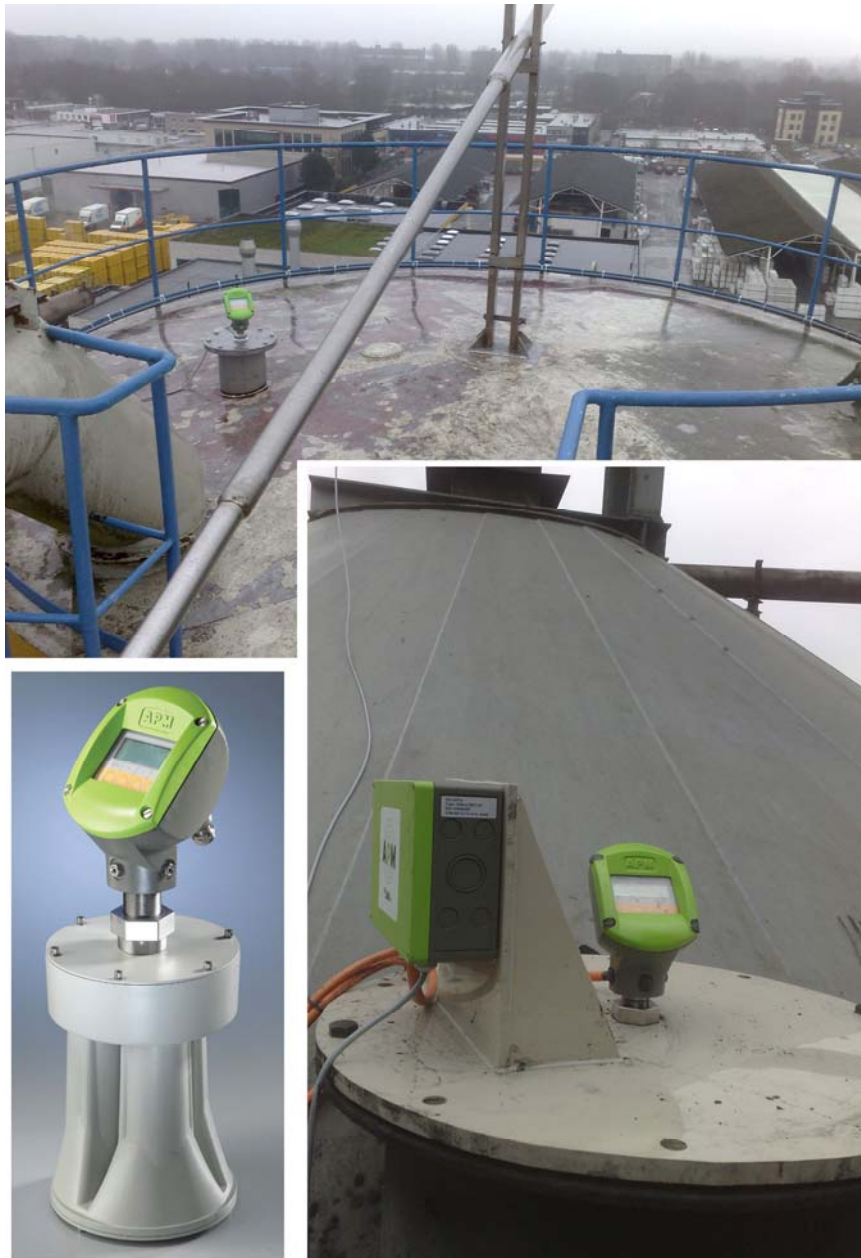
The 3DLevelScanner (left), installed on large silos, for cement (top), and together with the APM 3DLinkPro for GSM communications anywhere in the world, for chemicals (Titanium Dioxide, right).
